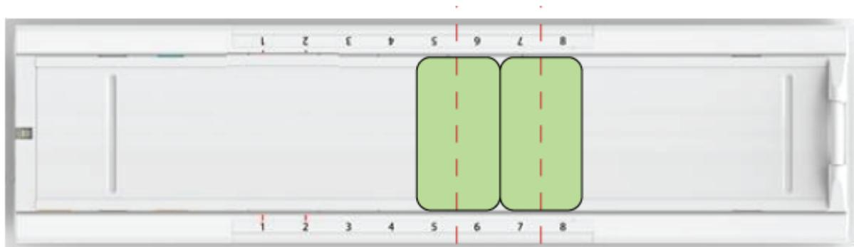
**Figure 4-4-4: Alignment of Two Water Phantoms with Rows 5-8 on Both Sides of the Bed**
